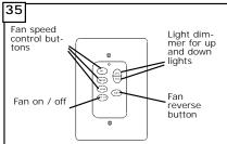
To control fan speed select from High, Medium or low speed buttons. To turn the fan off press the Fan on / off button. To dim upper lights press and hold U/L botton. To dim Lower lights press and hold D/L button. To turn off either up or down light press and quickly release either U/L or D/L button. Press button marked REV to reverse the rotation direction of the fan blades. blades
